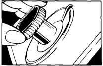
**C.** Start the washer by pulling out the Control Knob. After filling, the washer will agitate for the selected number of minutes.
